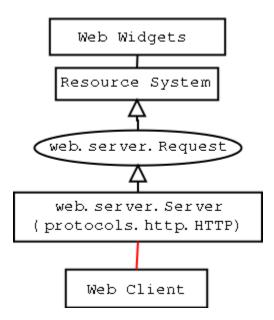
When the Web Server receives a request from a Client, it creates a Request object and passes it on to the Resource system. The Resource system dispatches to the appropriate Resource object based on what path was requested by the client. The Resource is asked to render itself, and the result is returned to the client.
